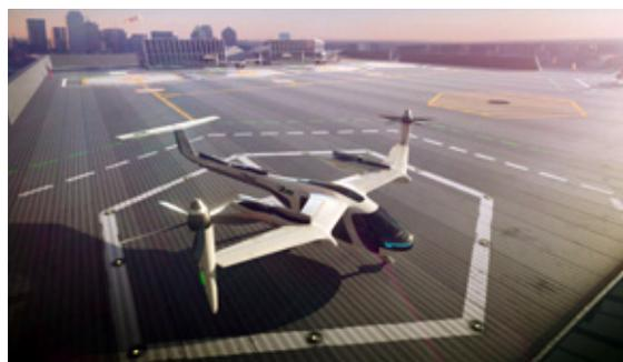
The resulting hybrid designs are completely novel and include both wings and multiple pivoting propellers. The technology community’s goal of industry disruption by moving fast and breaking things may work well when developing smartphone applications, but it becomes deeply problematic when the product involves human flight. Under federal law, the Federal Aviation Administration (FAA) must certify new aircraft designs and avionics systems.
